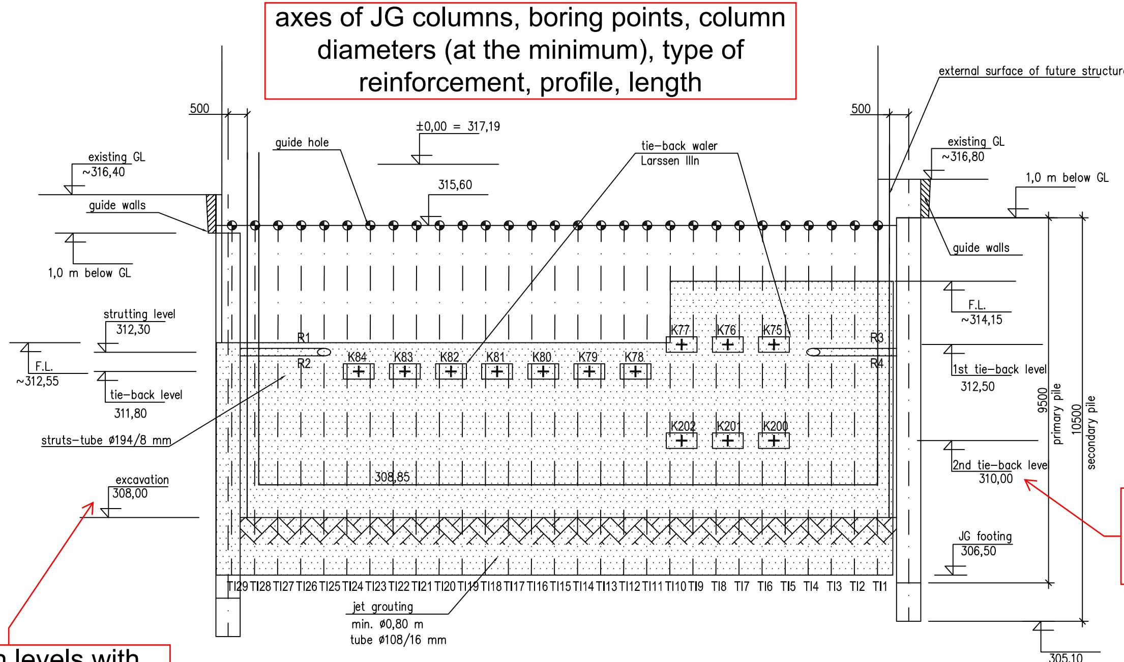
excavation levels with respect to stages of construction of the JG walls
