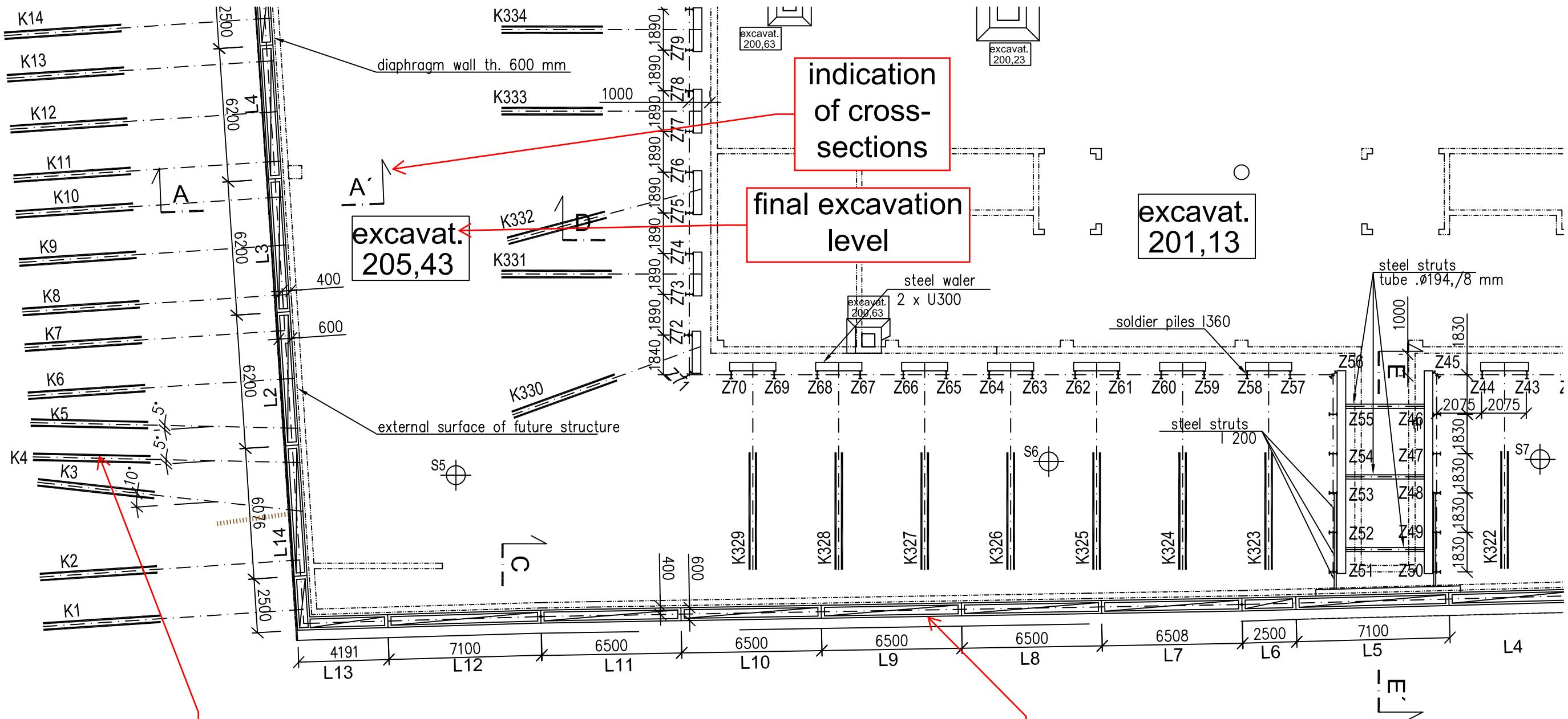
locations of anchors, free and fixed lengths / roots lengths, numbering of anchors, horizontal inclination to perpendicular of axis of the wall, if needed due to boring obstacles
