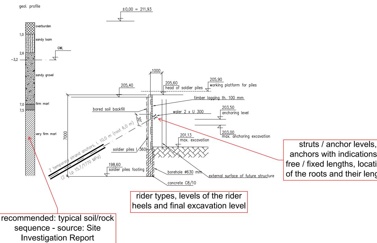
anchors with indications of free / fixed lengths, locations of the roots and their lengths
